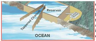
can then be channeled into a catch basin or used directly to spin turbines. There are no big commercial wave energy plants, but there are a few small ones. Small, on-shore sites have the best potential for the immediate future; they could produce enough energy to power local communities. Japan, which imports almost all of its fuel,
